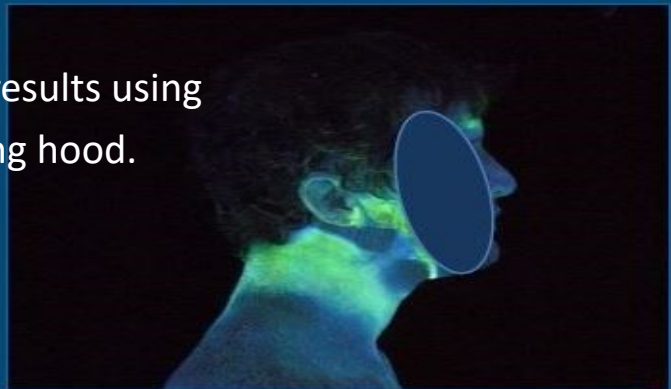
POST FAST Test results show dramatic contamination of the neck through standard hood after exposure to Fluorescent soot-like particulates.
